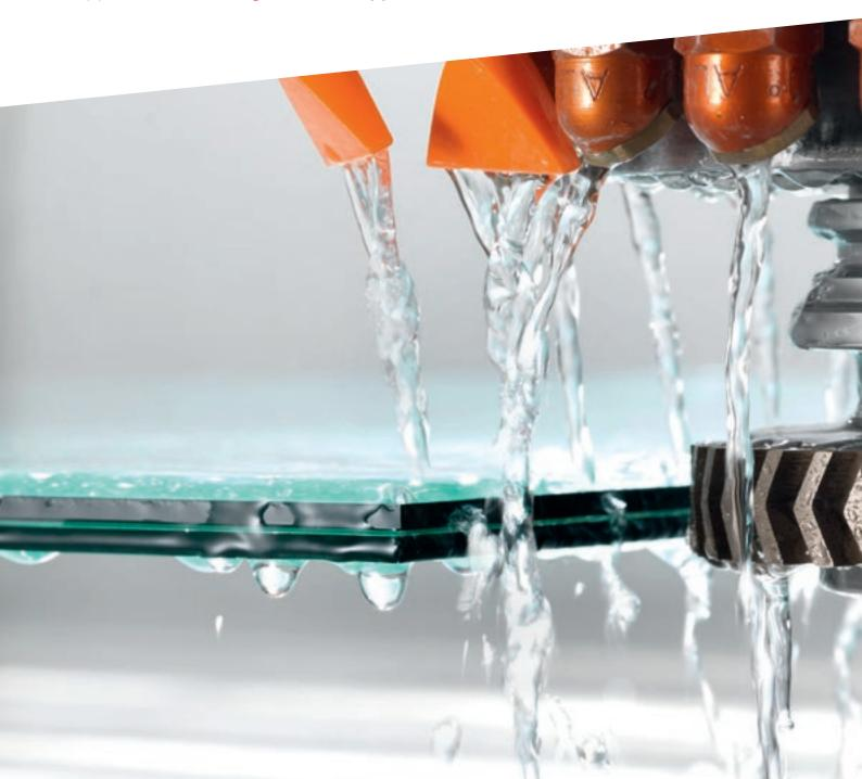
Chevron is the Diamut solution for laminated glass; The new profile is designed especially to optimise removal of plastic film and guarantee removal capabilities that have never been achieved before. In comparison to standard tools, the new V-shaped design also limits and delays the classic cutting at the centre of the groove caused by the plastic film which affects the performance of the tool.
